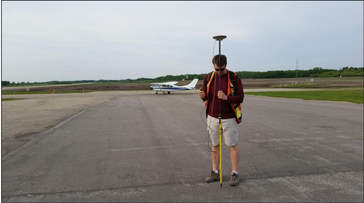
**Figure 8:** Example of Ground Check Point Collection
