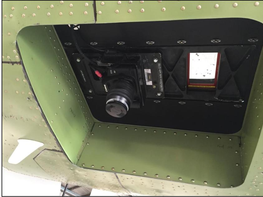
**Figure 3 : Camera Mounted on Piper 31 Navajo**
