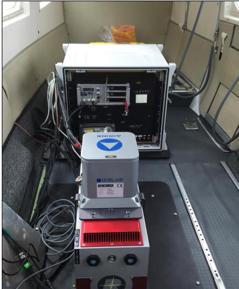
**Figure 2 :** Q780 Laser, IMU and Computers Mounted in the Piper 31 Navajo
